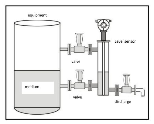
Generally speaking, the installation is very easy and simple. Only need to thead it on the top of tank by installed by flange which is required by the customer and nominated before producing. Of course when use flange, you need use bolts to fix it well and tightly, better add an sealing washer between flanges connection.
