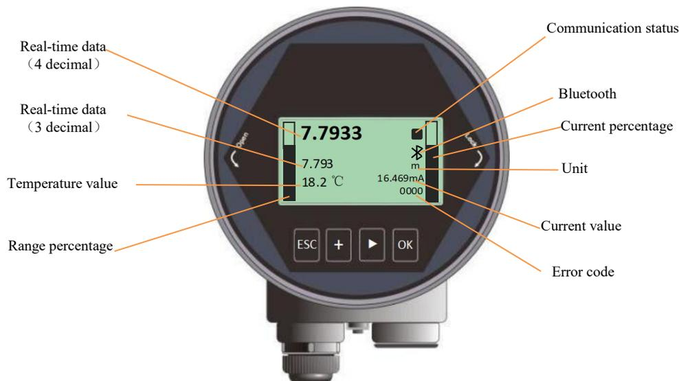
(1)Real-time data: Real-Time measurement result, which is converted from the distance between sensor and surface of medium.
