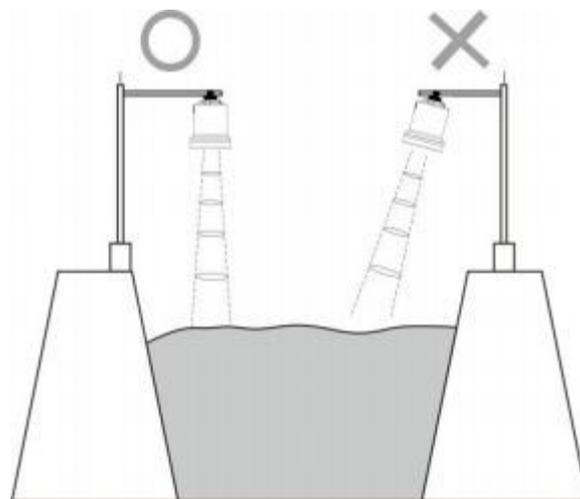
Fig. 4- 1 Diagram of the instrument installation location
