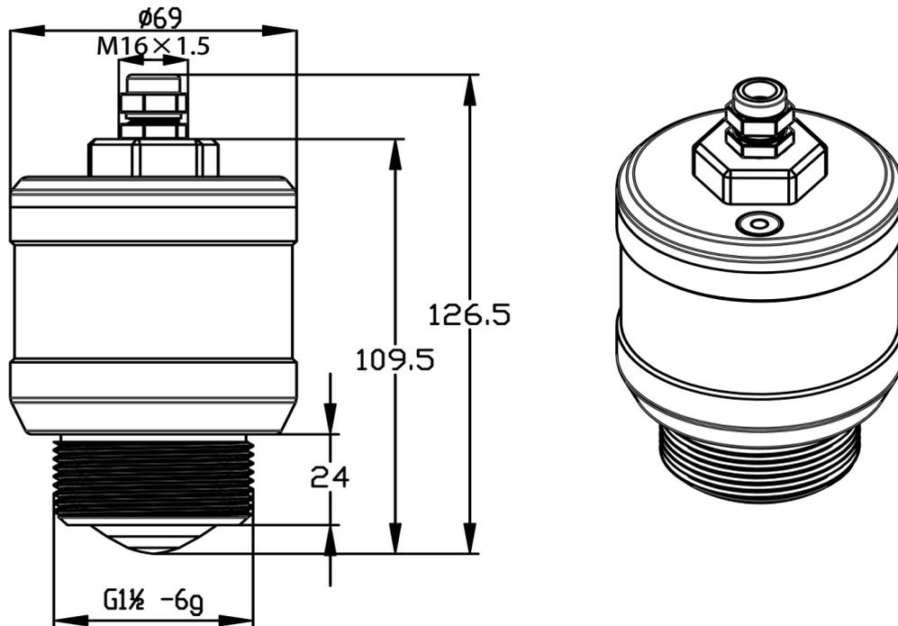
Fig.3- 1 Diagram of instrument structure size
