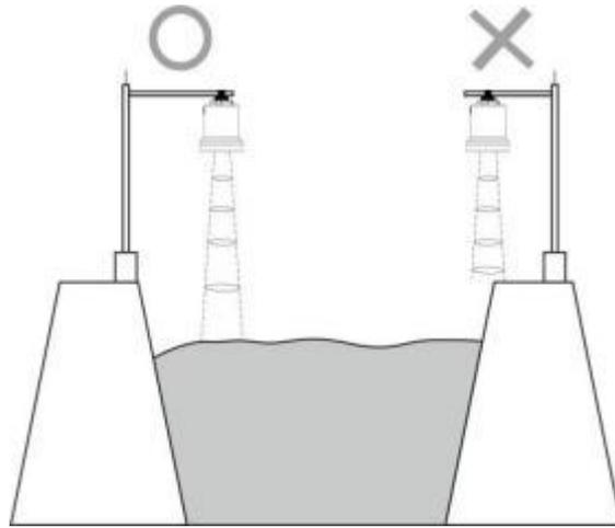
Fig. 4-2 Diagram of the instrument installation location
