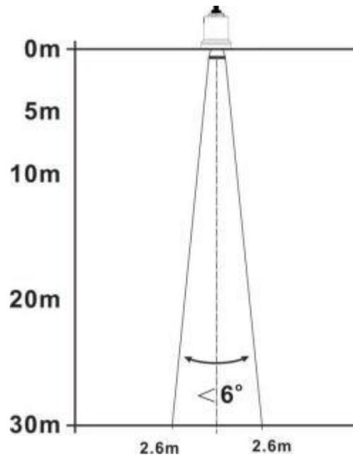
Fig.9 - 1 Diagram of the space geometry of the radar beam of the instrument
