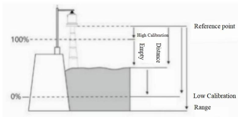
Fig.6– 1 Low Calibration interface and definition
